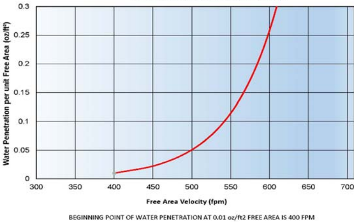
WATER PENETRATION - 2210 / 2215 15 MINUTE DURATION, TEST SIZE 48" X 48"
